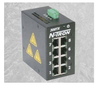
operating environmental specifications to meet the harsh needs of the industrial environment. For cost savings and convenience the 308TX can be DIN-Rail mounted alongside Ethernet I/O or other industrial equipment.
